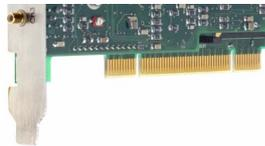
The cards with PCI/PCI-X bus connector use 32 Bit and up to 66 MHz clock rate for data transfer. They are 100% compatible to Conventional PCI > V2.1. The universal interface allows the use in PCI slots with 5 V I/O and 3.3 V I/O voltages as well as in PCI-
