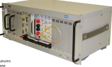
The 40-908 chassis is supplied fitted with three 55cfm fans to ensure efficient cooling of the chassis and modules.
