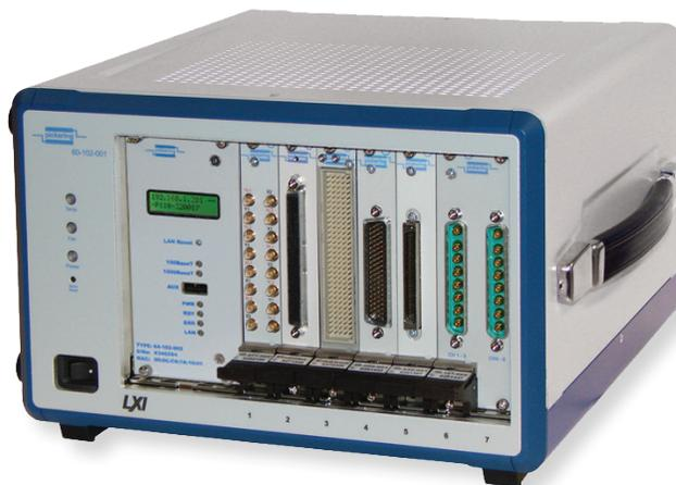
The 60-102B is fully compliant with the LXI Standard 1.4 and supports Pickering Interfaces 3U PXI switching and simulation modules. Each module is supported as though it is an LXI compliant device, complete with a driverless soft front panel that provides complete control of the module functions. The 60-102B supports up to 7 off 3U modules and is equivalent to an 8 slot PXI chassis.
