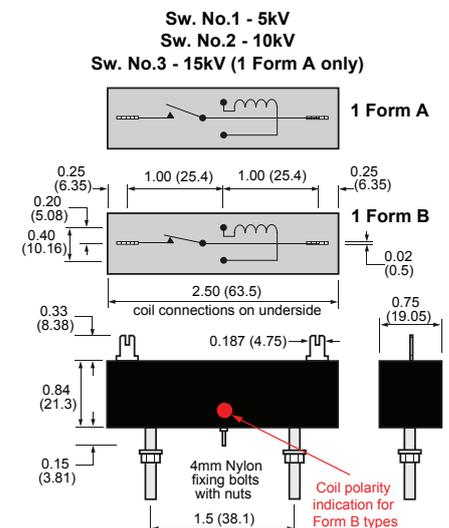
**Important:** For all Form B types, the correct coil polarity must be observed. The positive connection is shown by the red spot on the package.
