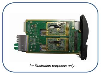
The High Sensitivity Receiver (HSR) has been designed for high loss environments where there are lots of splices/interconnects or low quality infrastructure. It mitigates or reduces the need for EDFAs, even working with CWDM and long distance systems where EDFAs are not available.
