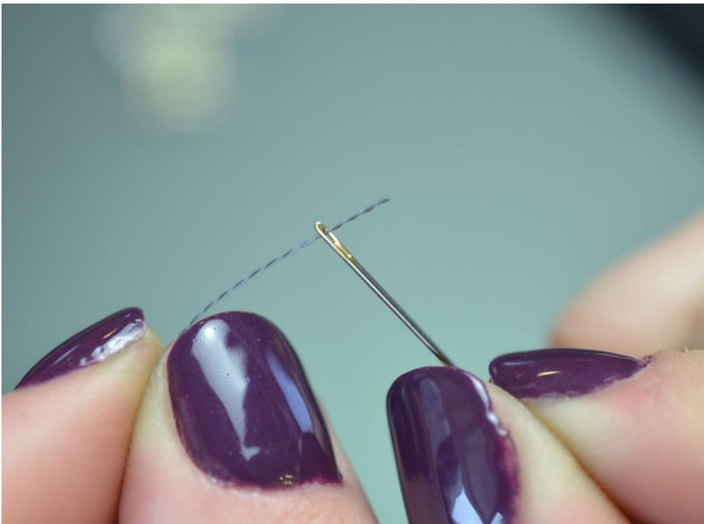
Grab a needle and test it's small enough to pass through the holes in the sequins. Thread up your needle with conductive thread, our 2-ply and 3-ply both are great for this purpose. [Check out our conductive thread guide \(https://adafruit.com/blog/2017/07/27/conductive-thread-guide/\)](https://adafruit.com/blog/2017/07/27/conductive-thread-guide/) to learn more about this stainless steel fiber.
