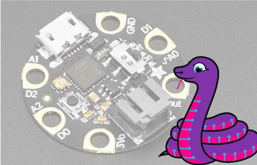
**GEMMA M0** boards can run **CircuitPython** — a different approach to programming compared to Arduino sketches. In fact, **CircuitPython** comes **factory pre-loaded** on **GEMMA M0**. If you've overwritten it with an Arduino sketch, or just want to learn the basics of setting up and using CircuitPython, this is explained in the [Adafruit GEMMA M0 guide](https://adafru.it/z1B) (<https://adafru.it/z1B>).
