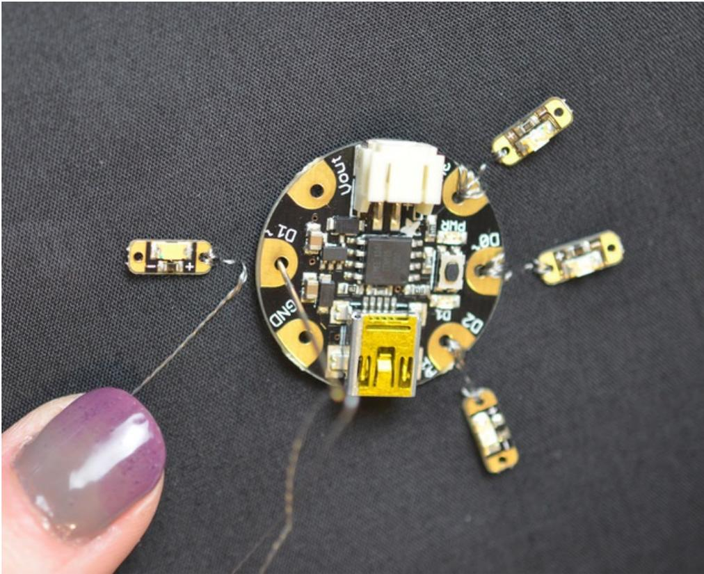
Stitch over to a digital or analog output on your microcontroller, and repeat the stitching process around the circuit board's pad.
