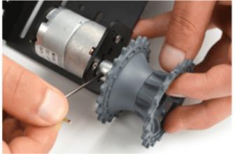
Step 6: Remove the track first, remove the excess part of the track, and measure the required track length.
