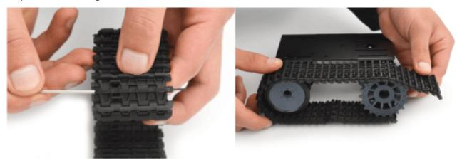
Embed the track pin into the track with a pair of pincers
