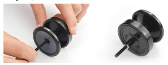
Step2: place the gasket on the bracket and insert the load-bearing wheel into the hole of the bracket; the other end is also fitted with a gasket, which is also locked with the M4 nut. Be careful not to screw the load-bearing wheel too tightly.
