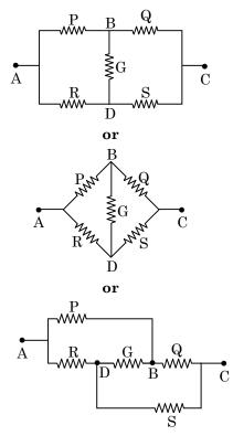
In a balanced Wheatstone bridge certain points are at same potential (see points B and D) and so no current flows through the resistor connected between such points (as the resistor G in above figures.) Therefore removing such resistors will have no effect on net resistance. Thus in a balanced Wheatstone bridge equivalent resistance can be drawn as follows:
