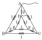
Sol. B and c are equipotential points and so are E and F. Here the circuit can be redrawn as shown in Figure.  $1\Omega$  and  $1\Omega$  in parallel sum up to 1/2W; 2W and 2W in parallel sum up to 1 W; 1/2W, 1 W, 1/2W in series sum up to  $1/2 + 1 + 1/2 = 2\Omega$ ;  $2\Omega$  and  $2\Omega$  in parallel sum up to =  $1\Omega$ .
